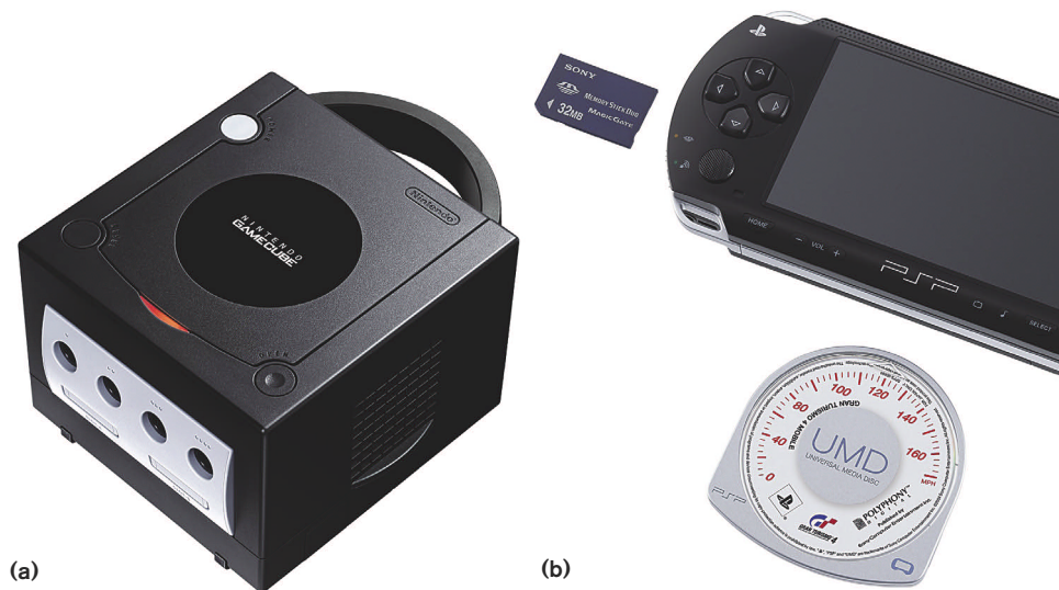
Figure 3 Nintendo's GameCube (a) and Sony's Playstation Portable (b) employ small-than-standard red-laser-media dimensions as one means of copy protection.
